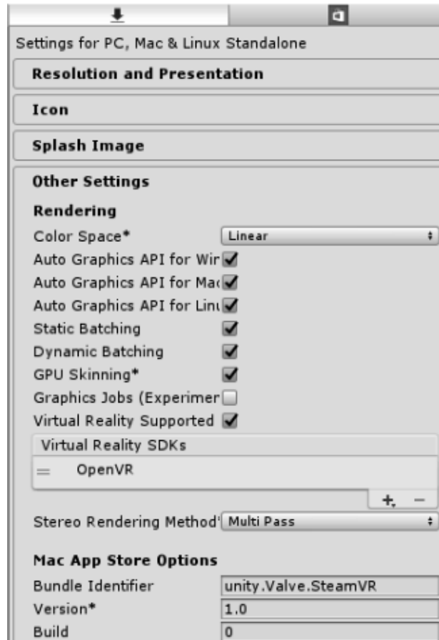
Figure. 1. Setting up virtual glasses for the Unity project: the Virtual Reality Supported option is enabled, OpenVR is added to the SDK list
